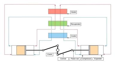
The Barton Engine is a heat engine; it converts heat (thermal energy) into mechanical energy, which can then be used to do mechanical work. Principally this will be to drive an electric generator, but it could instead, for example, drive an air compressor.
